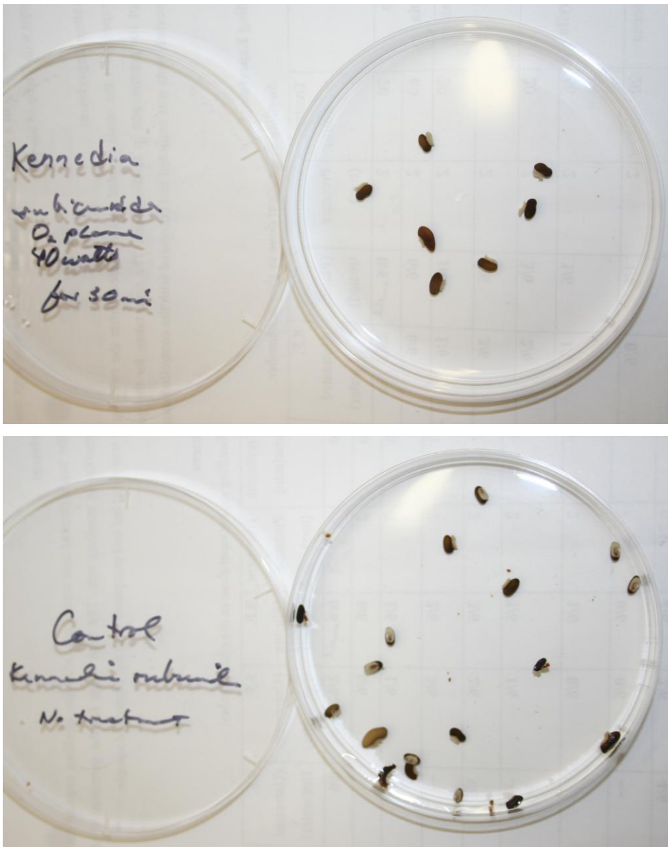
Figure 4. Seeds of Kennedia rubicunda that had been oxygen plasma treated (top) or not treated (bottom), after immersion in room temperature water for 24 hours.
