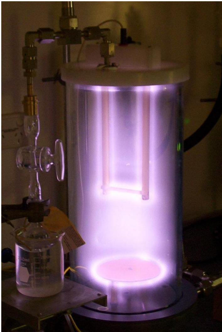
Figure 1. A gas plasma inside a glass chamber. The seeds are placed on the round table (diameter 90 mm).
