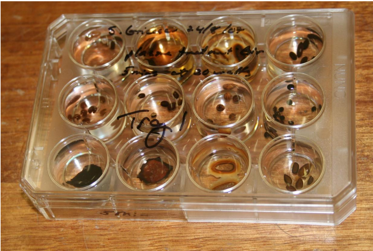
Figure 2. Experimental setup for soaking plasma treated and control seeds for 24 hours.
